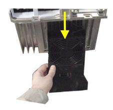
Pull down on the fan assembly. The fan and the fan guard will slip out of the heat sink in one piece.
