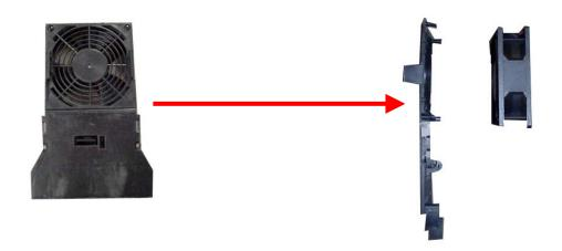
Use a screwdriver to pry the guard off of the fan. Use caution not to break the prongs that hold the two together. Simply install the replacement heatsink fan by reversing the steps in this guide.
