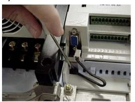
Disconnect the 24VDC power lead for the fan. It connects to the power board at the location shown above.
