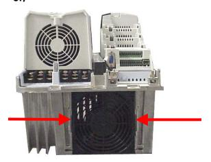
Position the drive so the fan is facing towards you. Push the retaining tabs in towards the center of the drive.
